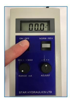
This device is desiged to operate 2-stage (pilot operated) servo valves with double coils with an amphenol connector P/N: MS3102-14S-2P.
